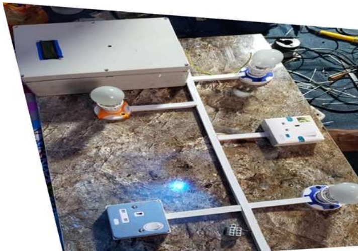
Figure 4: The developed model of automated power control system with accessories
